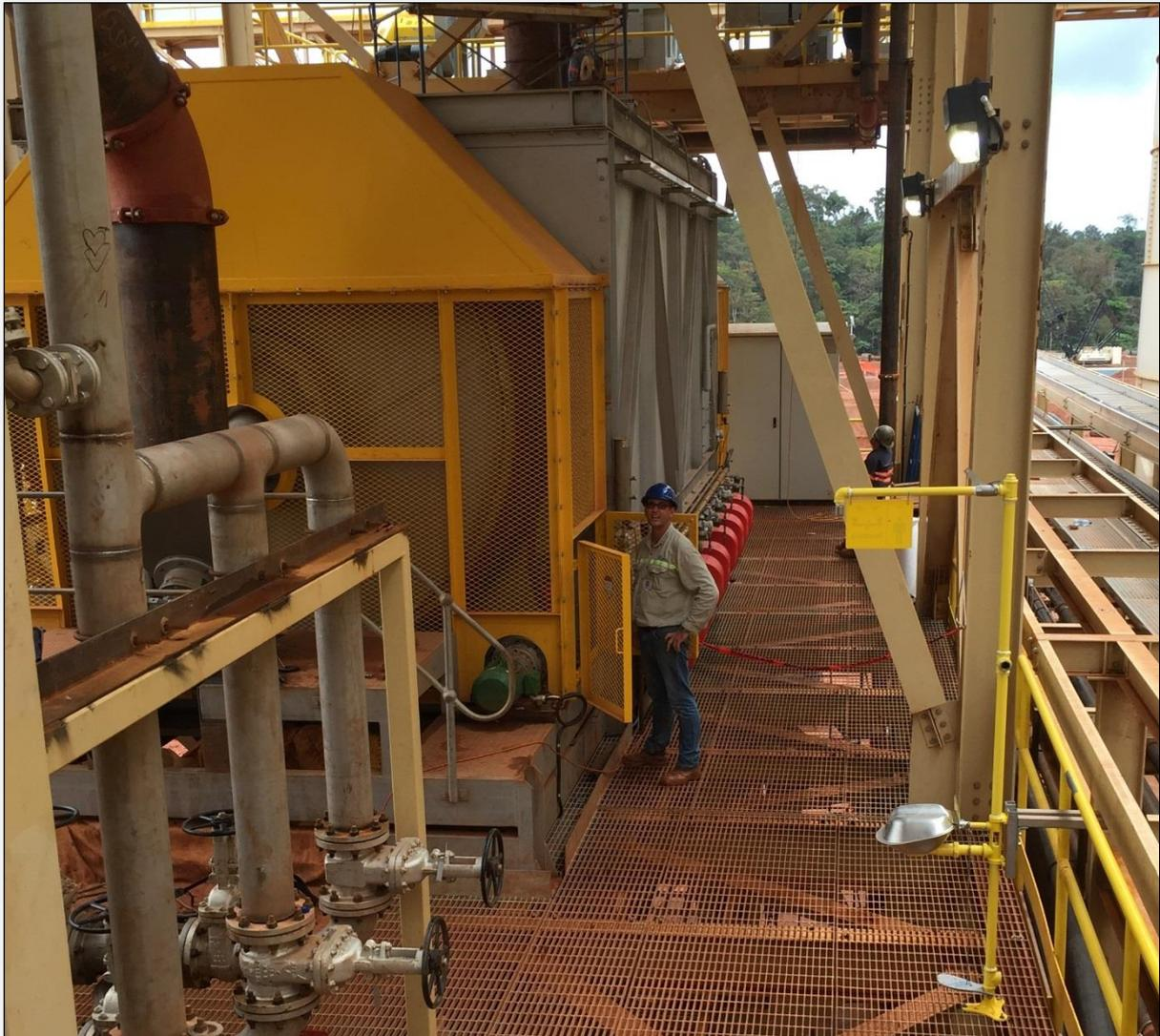
**1700 kg/h Diesel fired carbon regeneration kiln**
