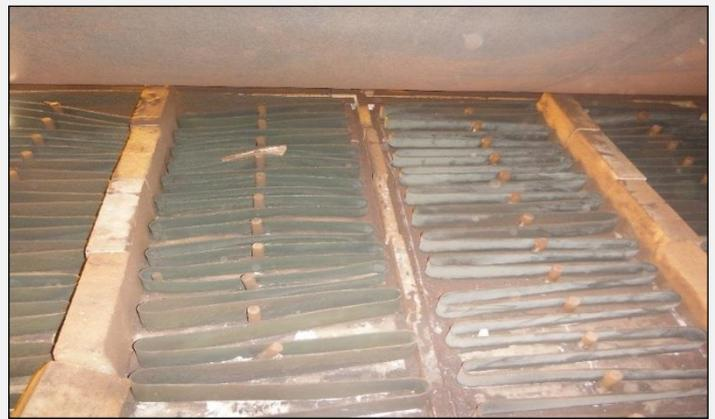
**Strip elements starting to fail after 2 months in operation – distortion of the steel elements can be seen**
