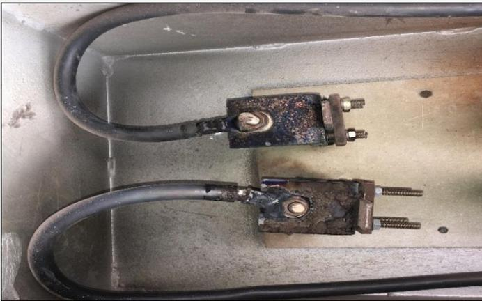
**Bus bar fatigue as a result of excessive heat from the element connection**
