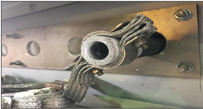
**Clamping arrangement on SIC elements
