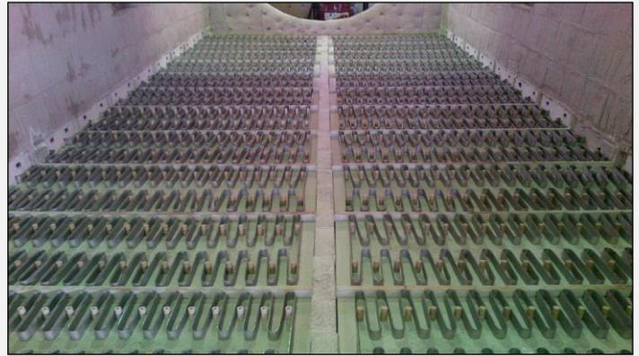
**New strip elements installed on the bottom of the kiln cabinet – if a retort failure occurs all elements would require replacement**
