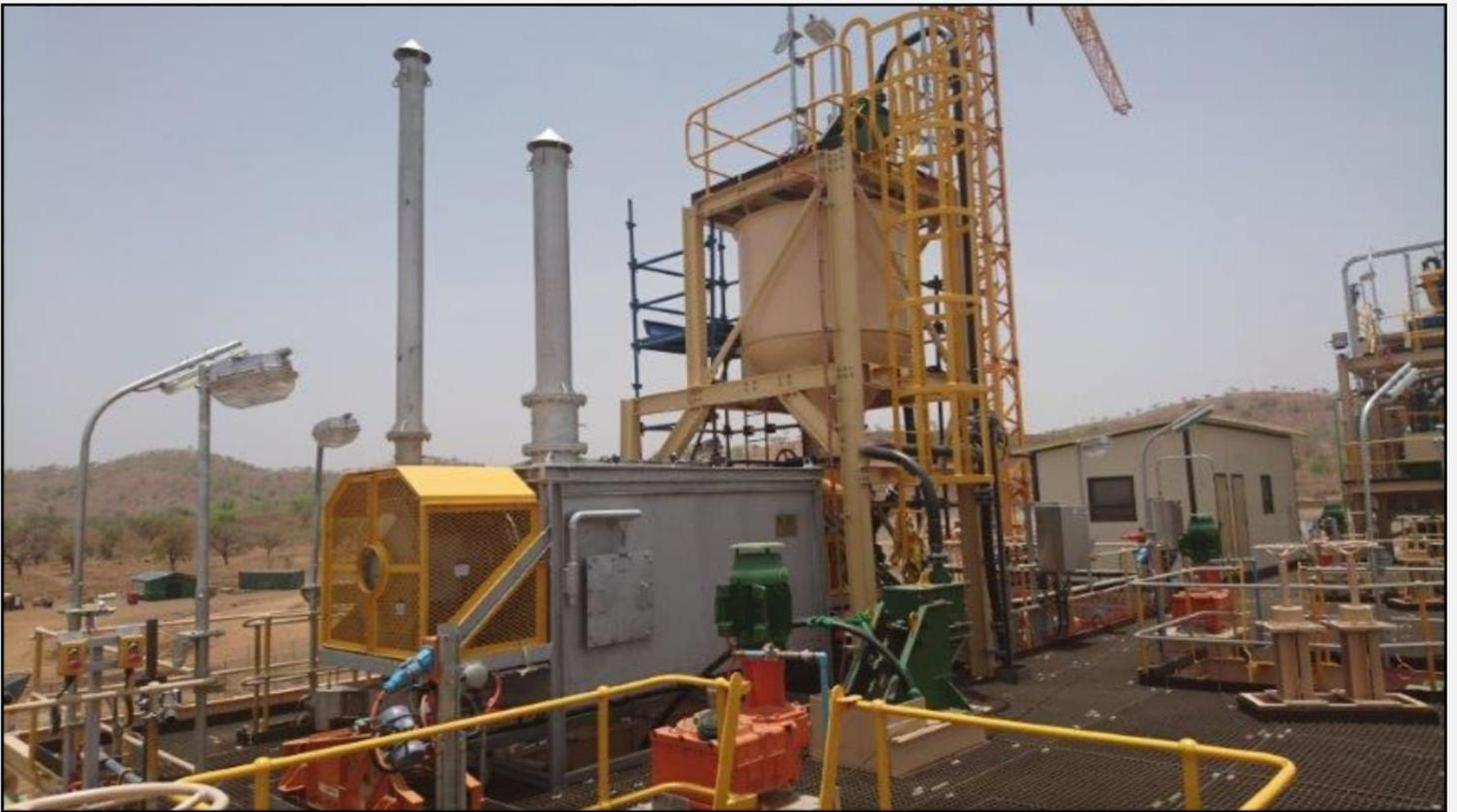
**100 kg/h Diesel fired carbon regeneration kiln c/w carbon holding hopper**
