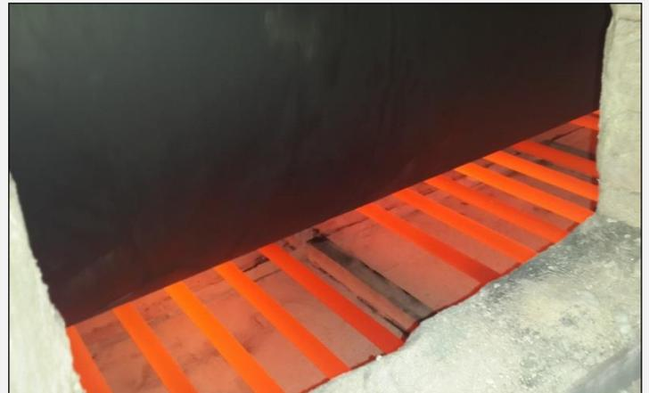
**Kemix SIC elements installed on bottom of the retort, operation at temperature**
