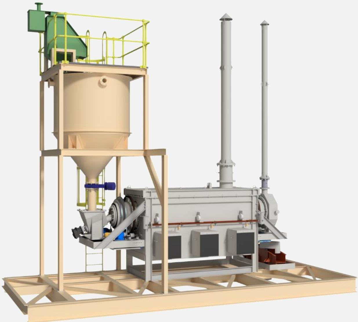
**3D Model of the 100 kg/h diesel fired carbon regeneration kiln c/w carbon holding hopper**
