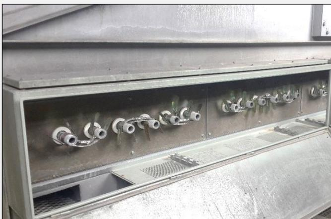
**Cold connections on bus bars when the kiln is in operation**
