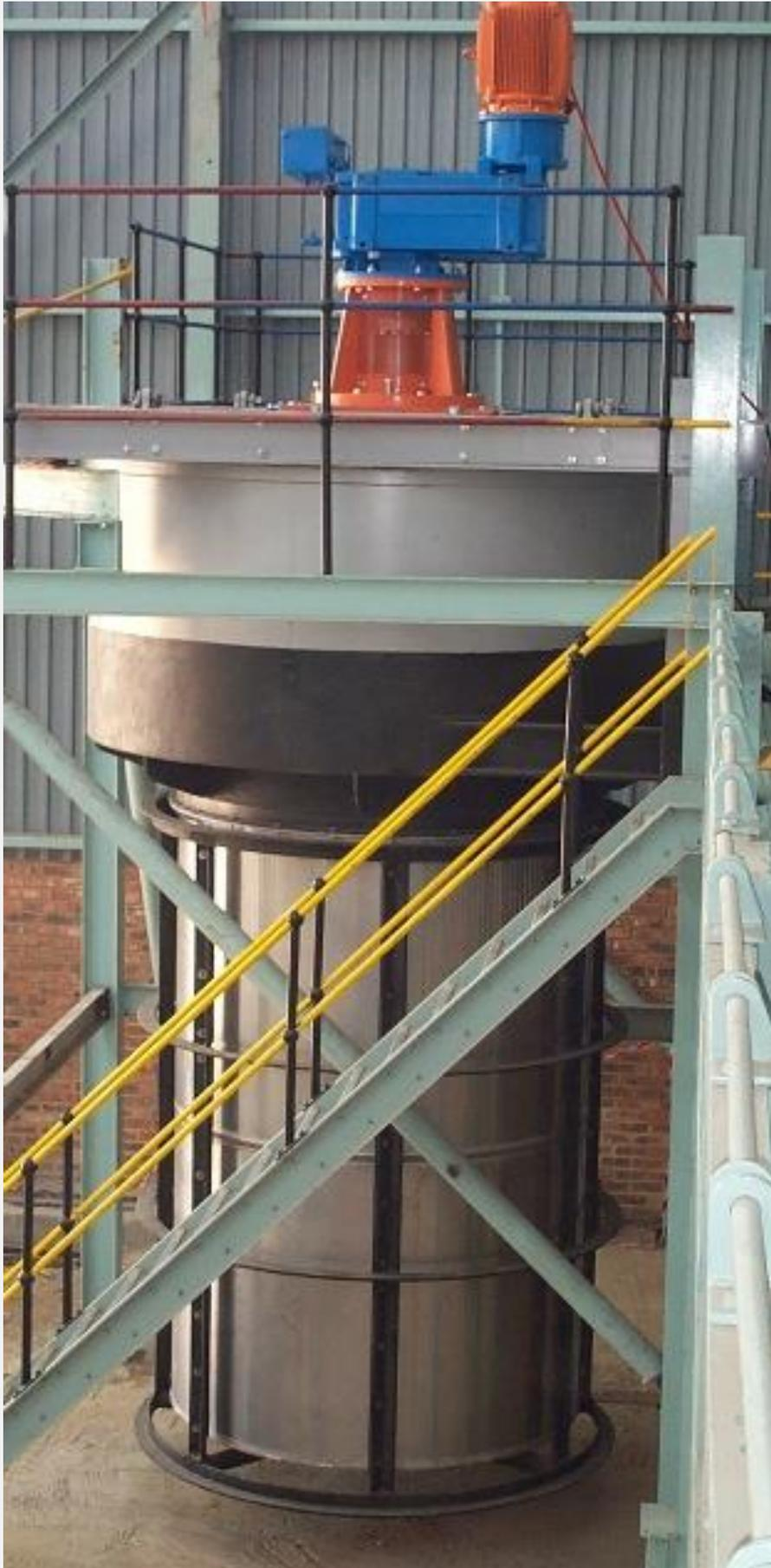
**Mineral processing separating pumping interstage screen (MPS 2030 (P))**
