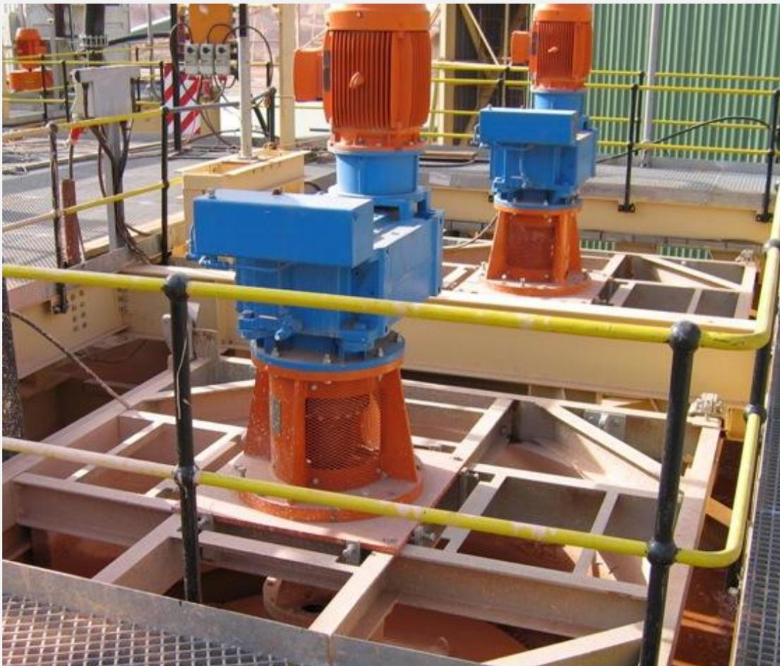
**Two mineral processing separating pumping interstage screens (MPS 2030 (P)) per tank**
